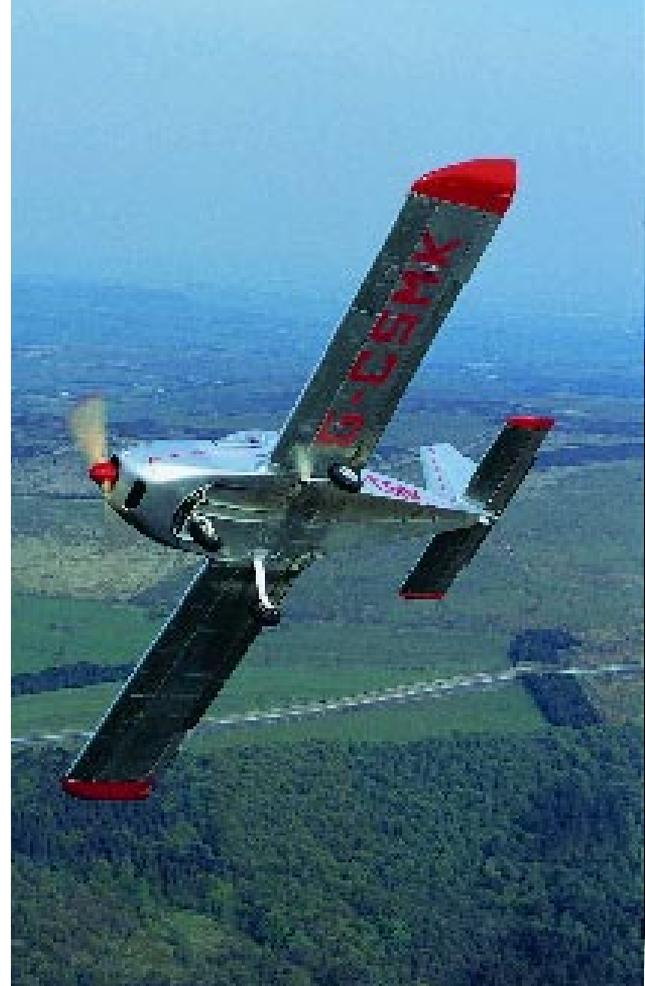
127kt. At about this point in a Dyn'Aero Ban-bi I had experienced a pitch oscillation through the stick which I found alarming. Not here. The Eurostar's little trim lever, which sits between the two seats, came in handy as the out-of-trim forces began to build. At this point the controls still felt great, and not heavy in roll or sensitive in pitch as with some others.
