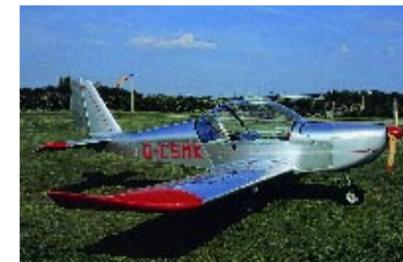
Thin anodised aluminium skin is traditionally manufactured; the lack of paint saves weight
