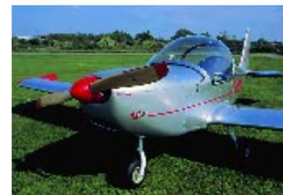
Closely cowled nose hides 80hp Rotax 912, perfectly adequate power for such a lightweight
