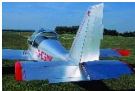
**Despite its diminutive stature, Eurostar is robust; well designed control surfaces give good handling**
